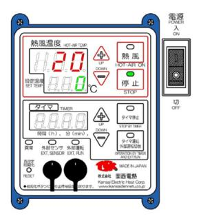
When you press the hot air switch, the hot air lamp (orange) lights up and hot air operation starts.
