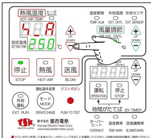
The changed discharge temperature upper limit set temperature controls the outlet temperature of the hot air generator when an external sensor is used, and is not the temperature of the safety circuit that stops the hot air generator due to a temperature abnormality. (Even if this change is made, the upper limit set temperature of the outlet temperature for abnormal temperature is not changed.) Therefore, the safety circuit will not operate at this changed temperature.
