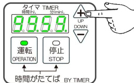
Time counting (Reduction of the setting time) is started (Flickering of the dot display), and hot-air operation is started when the time counting becomes to "00.00.". And, HOT-AIR lamp (Orange) is flickered during time counting, and the lamp changes to lighting after hot-air operation was started.
