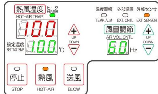
\* Barn out operates and operation is not started if the external sensor is set up in condition the external sensor is not connected (Refer to P14 of Operation manual Total adition).
