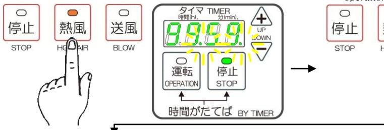
Cooling operation (Blow operation) is stopped when the time counting becomes to "00.00.", and BLOW lamp (Green) is flickered.
