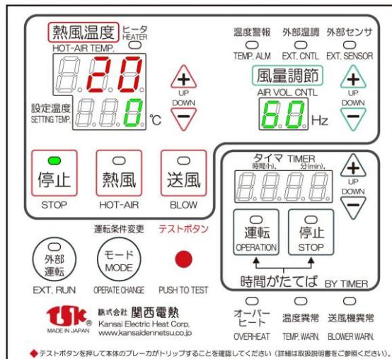
\* 2nd thereafter, the setting value of the previous time is displayed to SETTING TEMP. and AIR VOL. CNTL.
