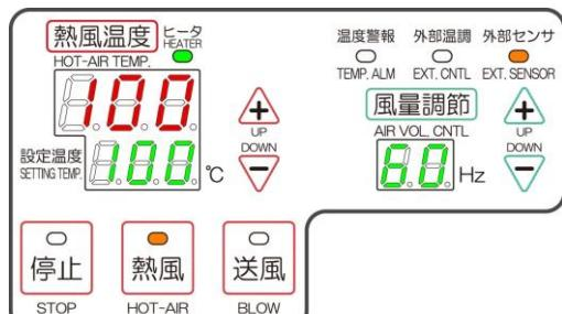
\* Hot-air generator is controlled by temp. that reached any early of temp. that was set up with the temp. controller of the outside or discharge setting temp. of the hot-air generator. So, please set up each temp. in consideration of the radiation of piping etc.
