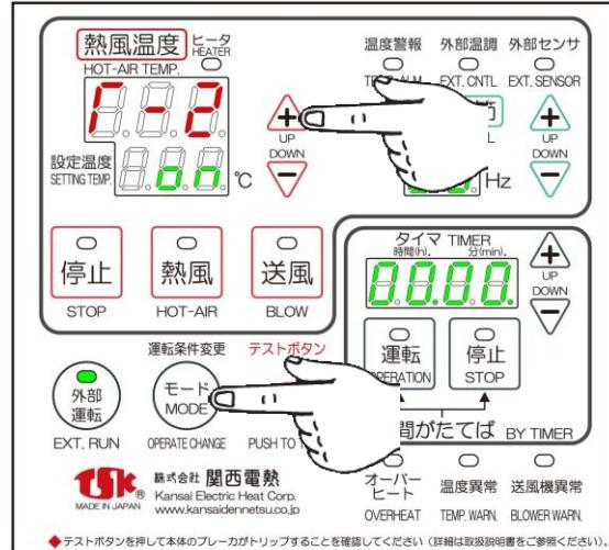
④ Please set up the hot-air operation time by pushing STOP BY TIMER.
