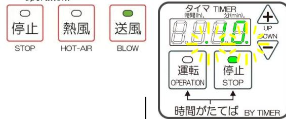
\* Timer operation is stopped by pushing STOP switch. (Timer setting is returned to the initial setting value.)
