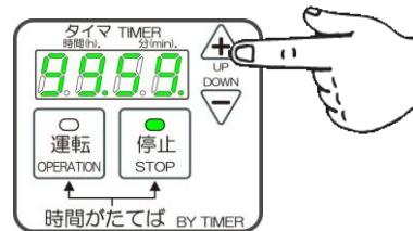
Cooling operation (Blow operation) is started by the timer after hot-air operation is stopped by the timer operation. And, BLOW lamp (Green) is lighted during cooling operation.
