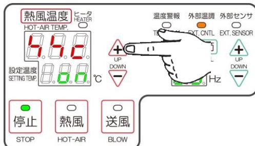
⑤ Please start hot-air operation after setting the optional temp. and air volume, and please start even temp. control by the temp. controller of the outside simultaneously.
