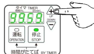
After the hot air operation ends via timer operation, the timer-controlled cooling operation (fan operation) will begin. The fan lamp (green) will also illuminate during cooling operation.
